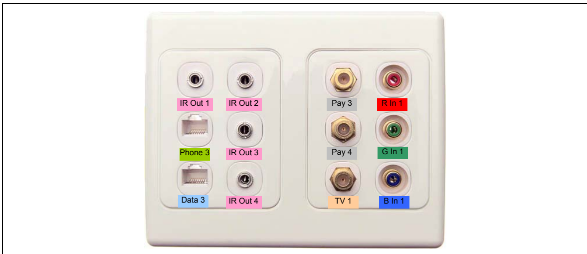
Two wall plates combined to provide remote InfraRed control of up to 8 devices, a Data Outlet (e.g. Personal Computer, Gaming Console, Media Receiver), Pay TV, Free to Air TV, and RGB inputs (e.g. from a DVD player or AV Receiver to a projector)
